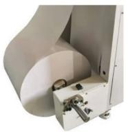
Offline roll to sheet cutting can be done with optional big unwinder unit (Chopin-350L model).
