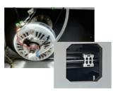
Fully automatic magnetic-powder tension break and semi-rotary slider type tension control system
