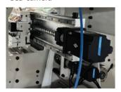
Strong X-Y driving by using thick lead screw actuators for heavy duty fast driving
