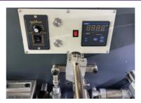
Heated matrix removal roller system with temperature controll for easy separation of strong-glued labels
