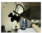
Matrix vision monitoring system to detect parts of weaker depth and adjust knife depth of each head automatically
